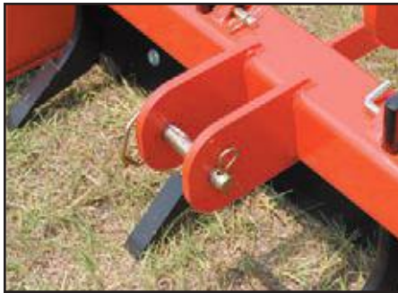
Scarifiers can rip soil up to 2 3/8" deep.
