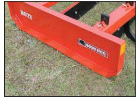
Full length, replaceable skids.
