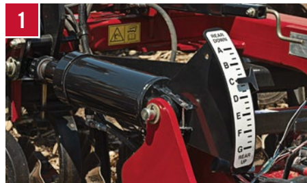
1 Hydraulic fore/aft control: maintain consistent agronomic output.
