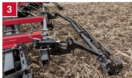
3 Crumbler pressure: achieve consistent clod sizing and finish.
