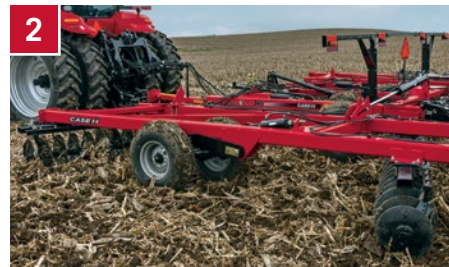
2 Disk gang depth: slice, cut and bury residue to the producer's desire.
