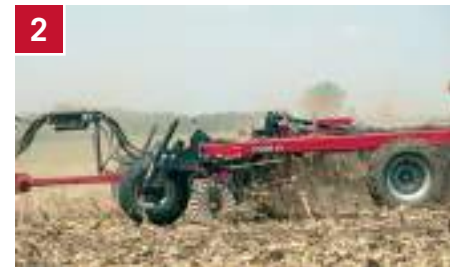
2 Disk Gang Depth: slice, cut and bury residue
