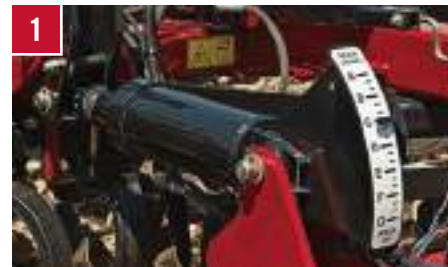
1 Hydraulic fore/aft control: maintain consistent agronomic output
