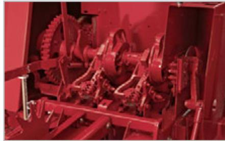
■ **Knotters** are gear-driven and built to wear for durability, consistent tying and low maintenance.
