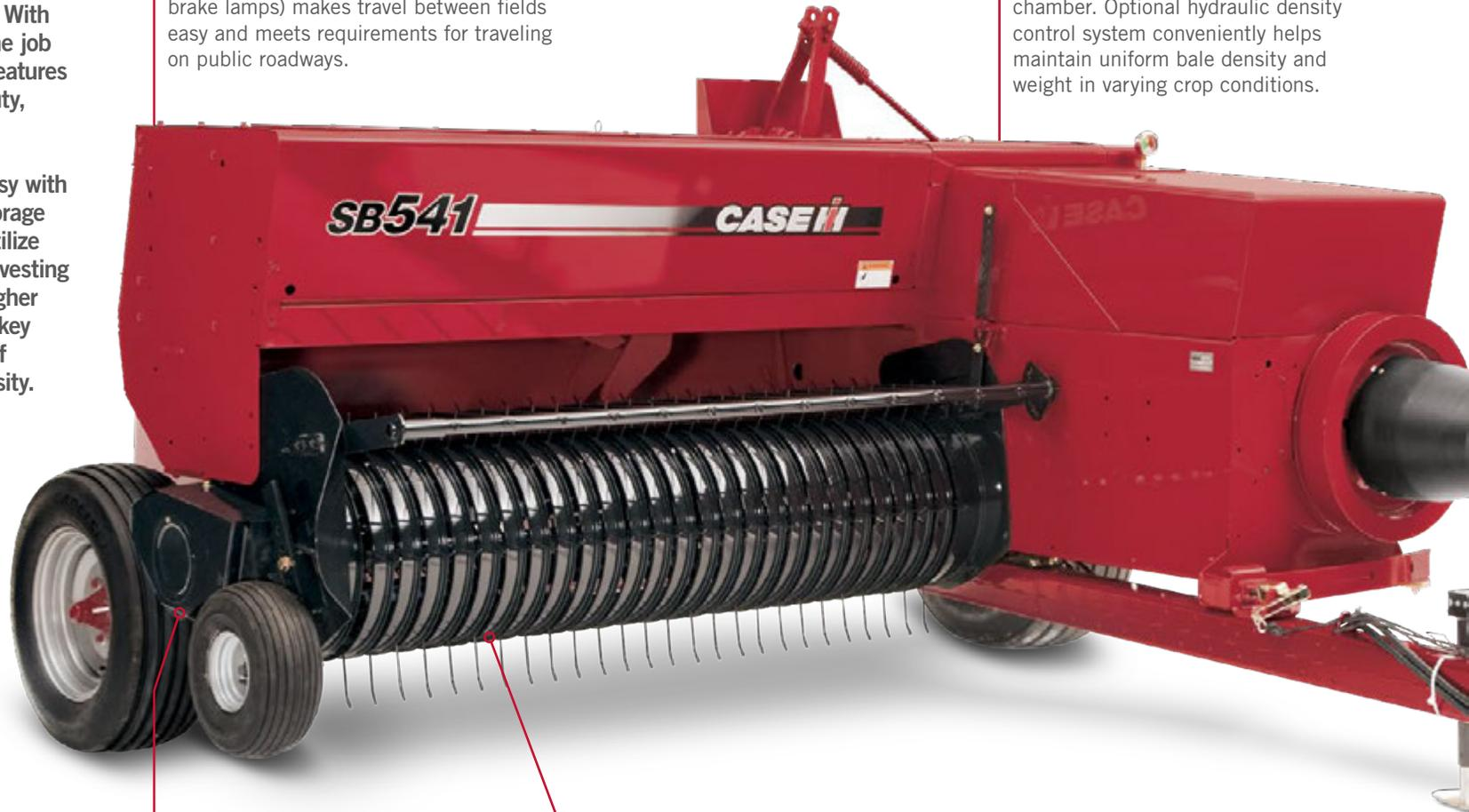
■ Pickup drive chain access shield gives easy entry to service points.
