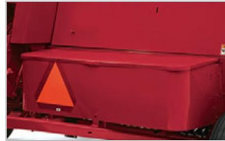
■ **8-twine bale box** allows for longer baling duration without rethreading increasing productivity in the field.
