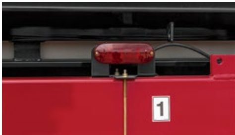
Tank full indicator lights.
