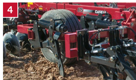
4 Shank depth: target the compaction layer
