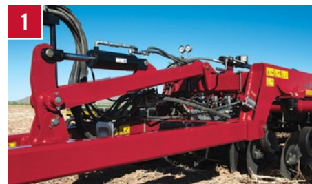
1 New hydraulic fore/aft positioning: maintain consistent agronomic output
