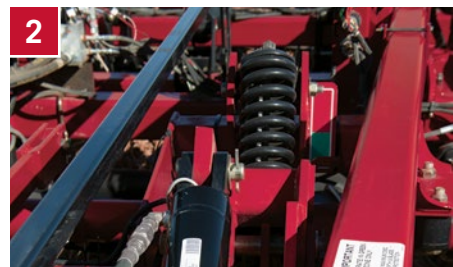
2 Disk gang pressure: reduce pressure on frame
