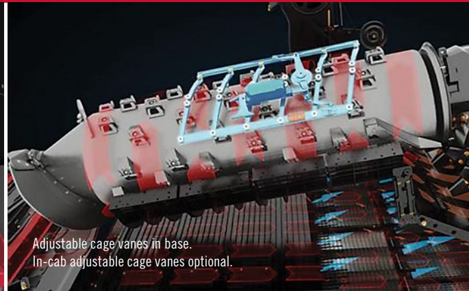
Adjustable cage vanes provide the operator the ability to optimize threshing and separating.
