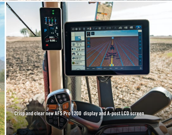
Redesigned MultiControl armrest and MultiFunction handle
